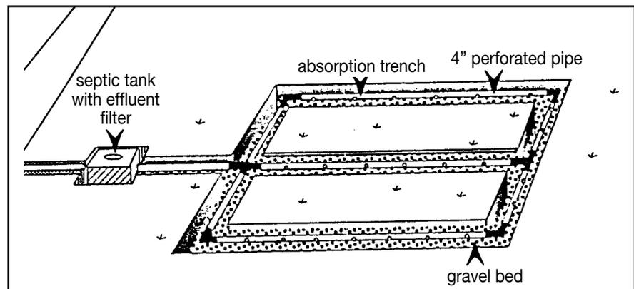
**Figure 1: Septic System with Effluent filter**—The Montana Waste Water Association requires effluent filters and risers of at least 21" diameter to w/in 6" of grade. Risers must have a shut off (float ball) built in so nothing will pass through if the filter cartridge is removed. When a riser is installed, it replaces the concrete lid and a new lid is placed at grade. Courtesy National Small Flows Clearinghouse \*
